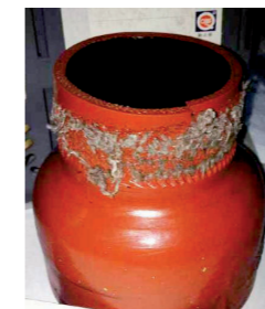
Damage to the rubber hose caused by the use of unedging hose clamp
